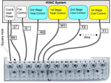
Figure 1 Single/Dual Stage HVAC Connections
