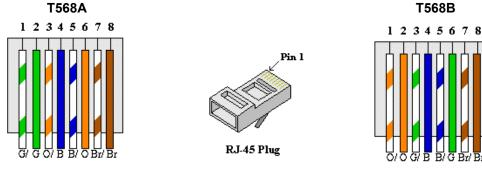
Table 5 describes the pinout assignments for the T568A and T568B wiring standards.
