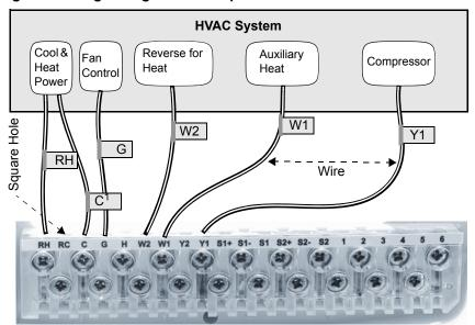
Figure 2 Single-Stage Heat Pump HVAC Connections
