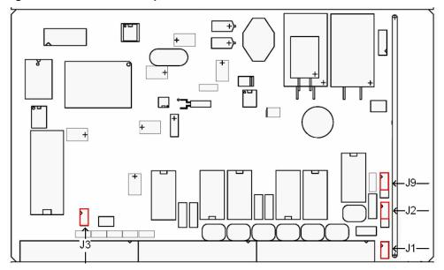
Prior to mounting the thermostat into the base plate, verify that the jumpers on the thermostat are configured for your application (see Table 6).
