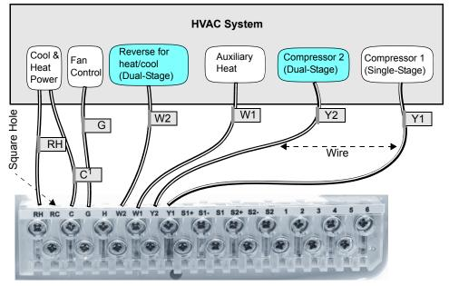
Figure 3 Dual-Stage Heat Pump HVAC Connections
